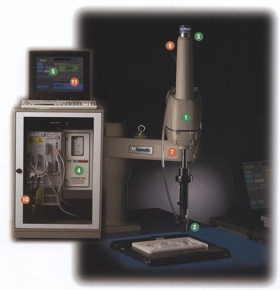
Finally, a fully programmed feeding and driving system as flexible as your current and future production needs demand. The Visumatic VIPer is offered in two standard configurations: a turnkey, stand alone assembly station or as a complete modular assembly component to meet the needs of machine builders and their customers.
